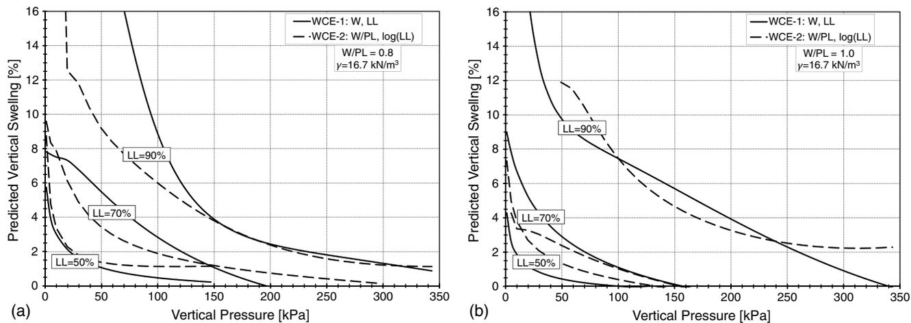
**Fig. 2.** Predicted vertical swelling versus vertical pressure for  $\gamma = 16.7 \text{ kN/m}^3$  as obtained from second-stage ANN models WCE-1 and WCE-2 for (a)  $W/PL = 0.8$ ; (b)  $W/PL = 1.0$
