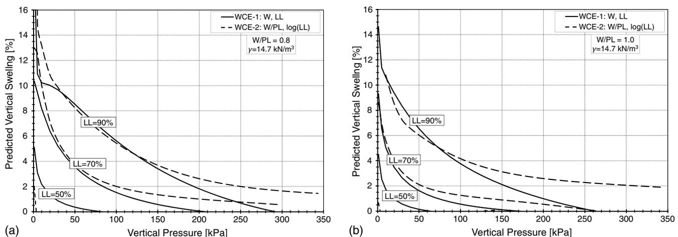
**Fig. 1.** Predicted vertical swelling versus vertical pressure for  $\gamma = 14.7 \text{ kN/m}^3$  obtained from second-stage ANN models WCE-1 and WCE-2 for (a) W/PL = 0.8; (b) W/PL = 1.0
