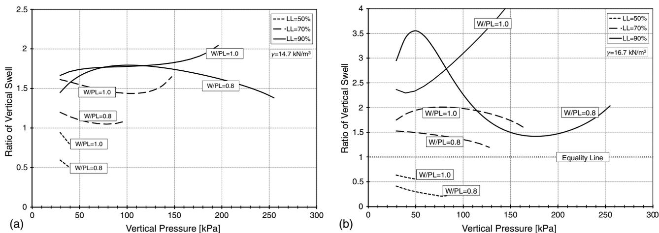
**Fig. 3.** Ratio of predicted vertical swelling, ANN WCE-1 model to ESC W-1 model, versus vertical pressure for (a)  $\gamma = 14.7 \text{ kN/m}^3$ ; (b)  $\gamma = 16.7 \text{ kN/m}^3$
