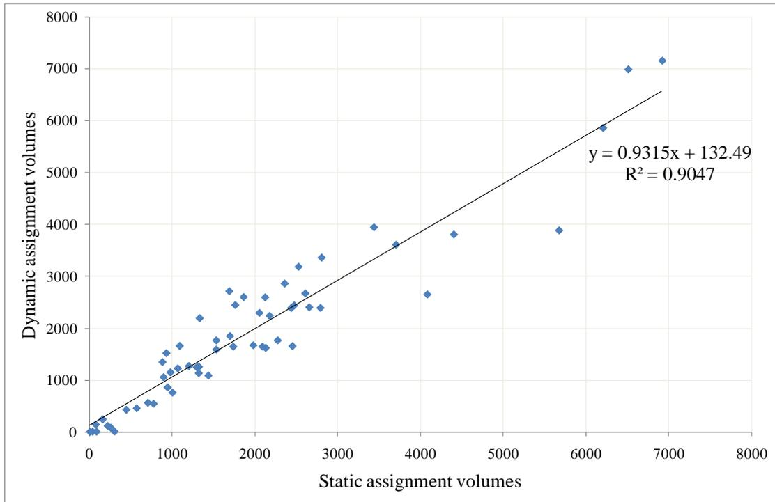
**FIGURE 18 Link flow comparison on screen lines – AM peak hour**
