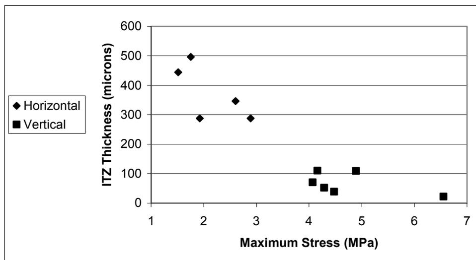
Figure 1 – Maximum stress versus ITZ thickness as measured using the gradient method
