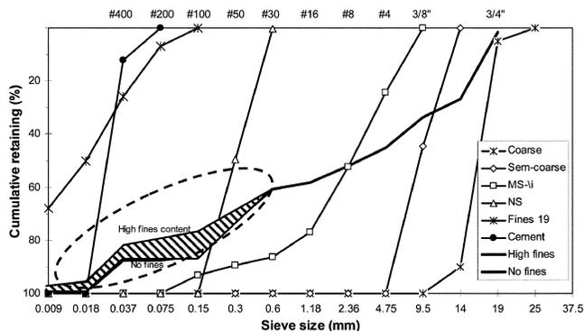
Fig. 1—Sieve analysis of tested aggregates, including Fines 19, cement, and their mixture limits.
