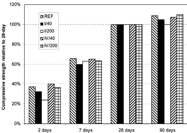
Fig. 10—Development of compressive strength for control and Series I and IV relative to their 28-day strength.
