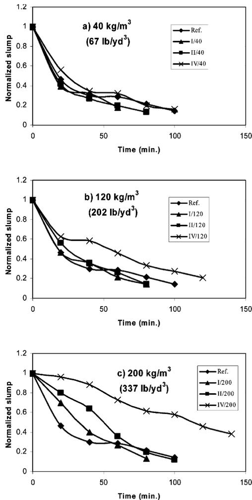
Fig. 7—Slump loss over time for various mixtures.
