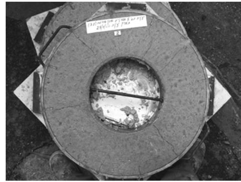
Fig. 8—Early-age cracking of Mixture IV/160.
