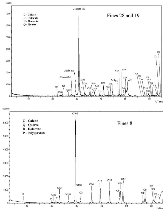
Fig. 2—X-ray diffraction of fines.
