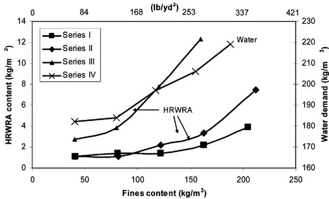
Fig. 6—Effect of fines on admixtures and water demand required for constant slump ( $1 \text{ kg/m}^3 = 1.69 \text{ lb/yd}^3$ ).
