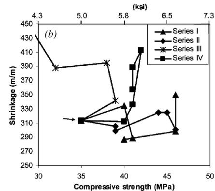
Fig. 13—Strength-carbonation: (a) strength shrinkage; and (b) relationships.
