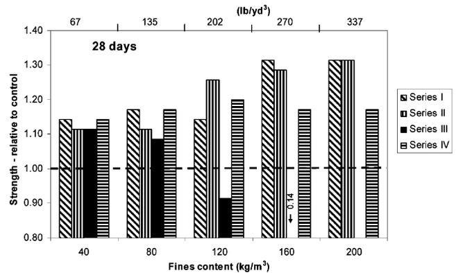
Fig. 9—Compressive strength at 28 days relative to control mixture.
