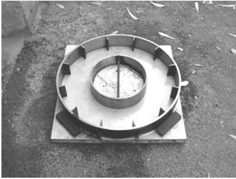
Fig. 5—Apparatus for detecting plastic shrinkage cracking.
