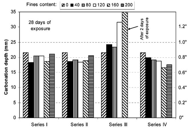
Fig. 12—Carbonation depth after 28 days of exposure to accelerated carbonation condition.
