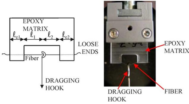
Fig. 1. Schematic diagram of drag out specimen and picture of spectra/epoxy specimen in the tensile holder.
