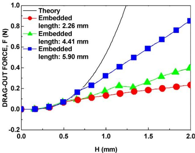
Fig. 3. The drag-out force  $F$  as measured with different embedded lengths. The predicted theoretical line (Eq. (4) or, equivalently, Eq. (6)) is shown for comparison.
