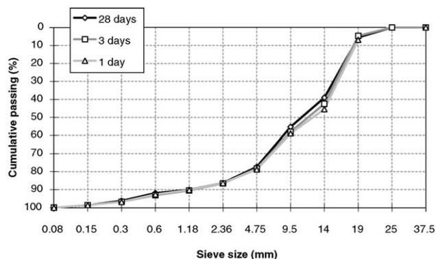
Fig. 1. Grading of the recycled aggregates crushed at various ages.
