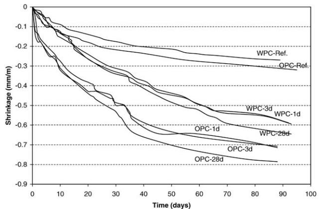
Fig. 6. Shrinkage of the new concrete made from white cement (WPC) and ordinary cement (OPC).
