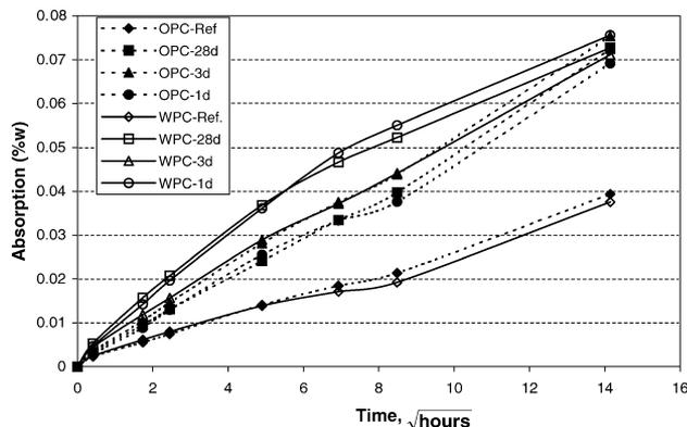
Fig. 5. Absorption rate of the recycled concretes and reference concrete.
