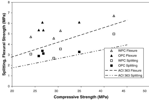
Fig. 4. Flexural and splitting strengths vs. compressive strength.
