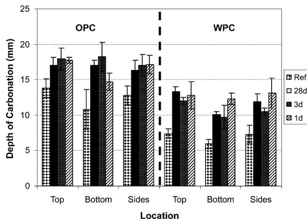
Fig. 7. Depth of carbonation at the different sides of the tested prisms after 7 days in the carbonation chamber.
