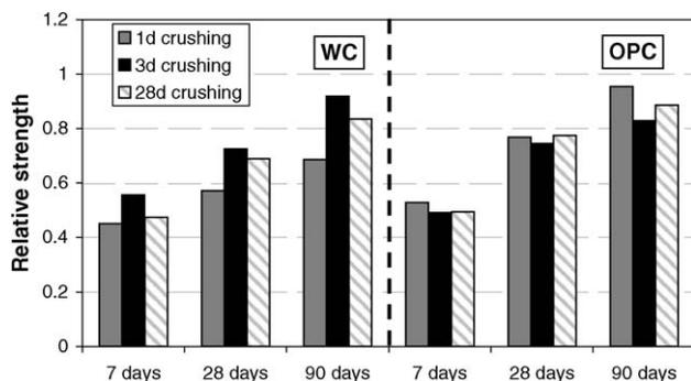
Fig. 3. The compressive strength of recycled concrete crushed at different ages relative to the reference concretes.
