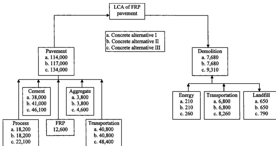
Fig. 3. Environmental load, in Eco-indicator 99 points, for the entire life cycle of FRP reinforced pavement
