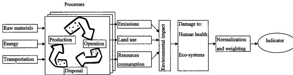
Fig. 1. Flow of environmental impact assessment of processes
