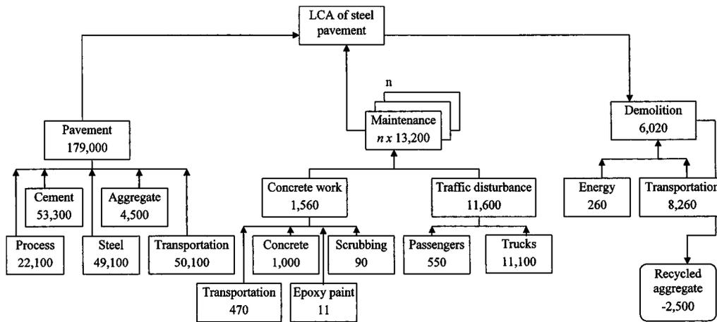
Fig. 2. Environmental load, in Eco-indicator 99 points, for entire life cycle of steel reinforced pavement
