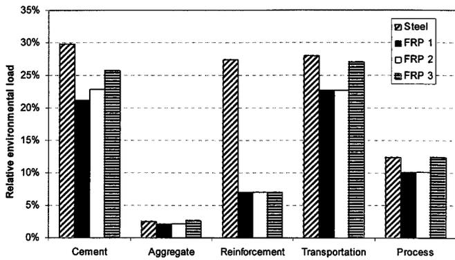
**Fig. 4.** Comparison of environmental load of pavement erection, using Eco-indicator 99 method, normalized to load of steel reinforced pavement
