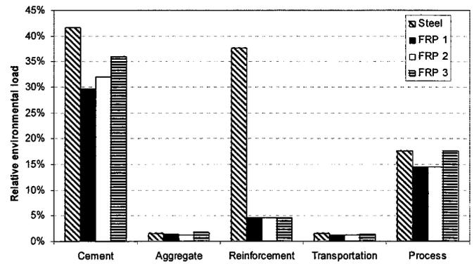
**Fig. 5.** Comparison of relative environmental load of pavement erection, using EPS 2,000 method, normalized to load of steel reinforced pavement
