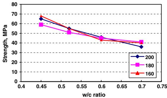
**Fig. 1** Effect of cement content (i.e. different levels of water contents of about 160, 180 and 200 kg/m<sup>3</sup> of concrete) on 28 days compressive strength
