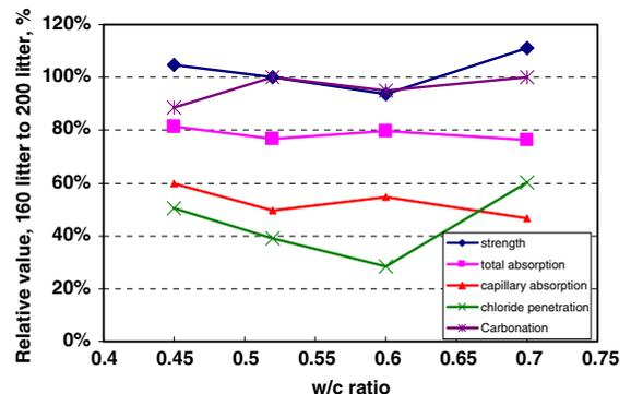
Fig. 10 The effect of cement content on the relative values of strength, total absorption, capillary absorption, chloride penetration and carbonation for mixtures with about  $160 \text{ kg/m}^3$  water content relative to mixtures with about  $200 \text{ kg/m}^3$  of water, i.e. cement content reduction of about 20%
