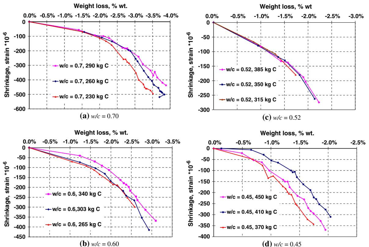
**Fig. 6** Effect of cement content on shrinkage—weight loss curves of concretes having the same  $w/c$  ratio but differing in their cement content. (a)  $w/c = 0.70$ , (b)  $w/c = 0.60$ , (c)  $w/c = 0.52$ , (d)  $w/c = 0.45$
