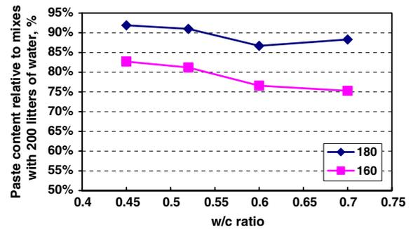
**Fig. 12** The paste contents in concretes with about 160 and 180 kg/m<sup>3</sup> of water relative to the 200 kg/m<sup>3</sup> water content concretes
