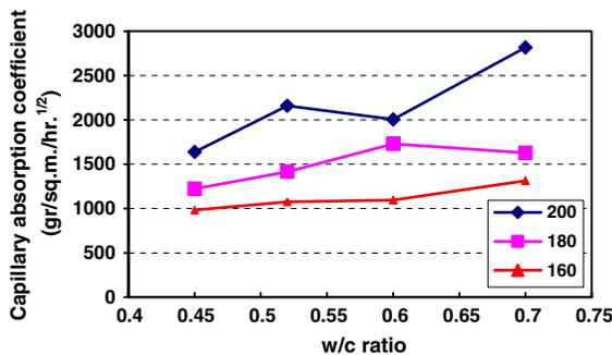
**Fig. 3** Effect of cement content (i.e. different levels of water contents of about 160, 180 and 200 kg/m<sup>3</sup> of concrete) on capillary absorption coefficient
