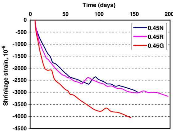
Fig. 8 The effect of admixture content and type on the shrinkage of  $w/c = 0.45$  paste (0.45 N—without admixture; 0.45R—with Rheobuild 2000 admixture; 0.45G—with Glenium admixture)
