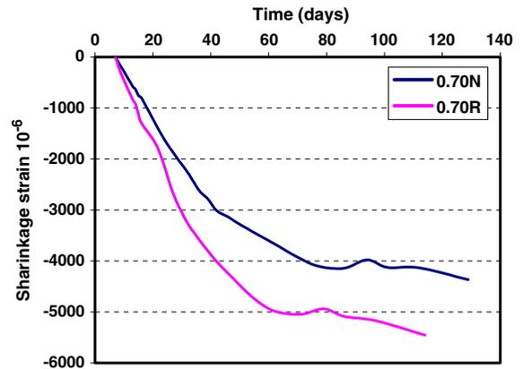
Fig. 9 The effect of admixture content and type on the shrinkage of  $w/c = 0.70$  paste (0.70 N—without admixture; 0.70R—with Rheobuild 700 admixture)
