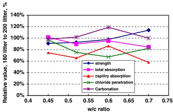
**Fig. 11** The effect of cement content on the relative values of strength, total absorption, capillary absorption, chloride penetration and carbonation for mixtures with about 180 kg/m<sup>3</sup> water content relative to mixtures with about 200 kg/m<sup>3</sup> of water, i.e. cement content reduction of about 10%
