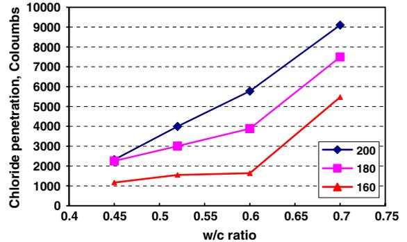
**Fig. 4** Effect of cement content (i.e. different levels of water contents of about 160, 180 and 200 kg/m<sup>3</sup> of concrete) on chloride penetration
