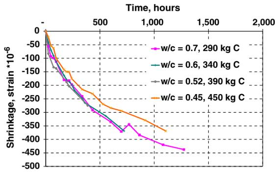
Fig. 7 Effect of  $w/c$  on shrinkage-time curves of concretes having a similar water content of about  $200 \text{ kg/m}^3$
