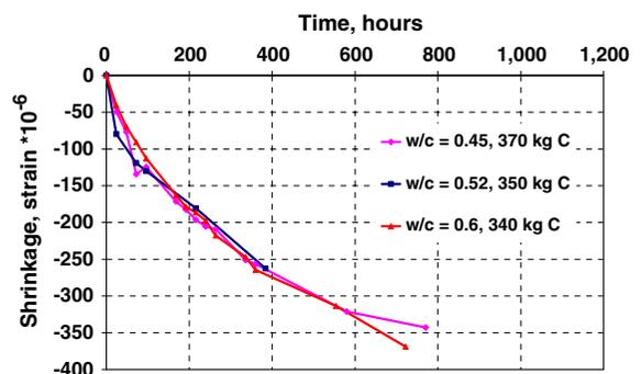
Fig. 14 Effect of *w/c* on shrinkage of concretes having a roughly similar cement content of about  $350 \text{ kg/m}^3$
