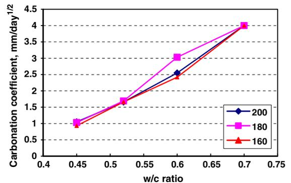
**Fig. 5** Effect of cement content (i.e. different levels of water contents of about 160, 180 and 200 kg/m<sup>3</sup> of concrete) on carbonation coefficient in accelerating conditions
