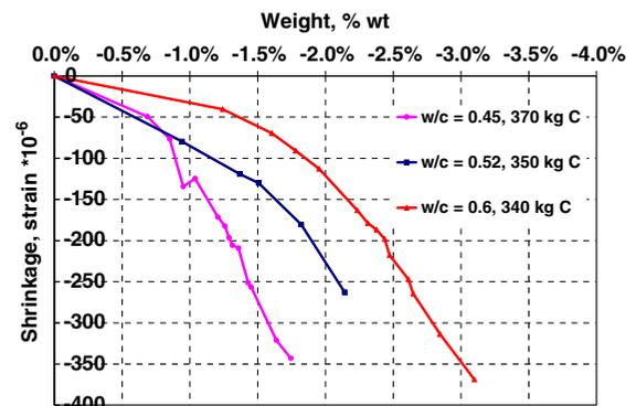
Fig. 13 Effect of *w/c* on shrinkage—weight loss curves of concretes having a roughly similar cement content of about  $350 \text{ kg/m}^3$
