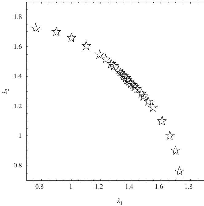
Fig. 1. Critical failure stretches.
